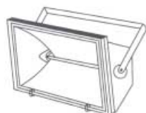
(a) Type B floodlight giving a fan-shaped beam
